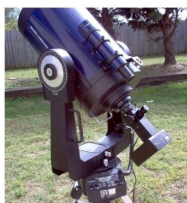
Figure 2: An example PEP-IR setup: the SSP-4 mounted on a 10" Meade LX200. The photometer unit fits into the standard 1.25-inch port at the Cassegrain focus.
