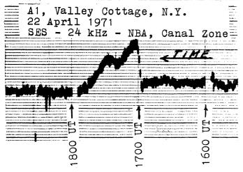
The first event on the 22nd, peaking at about 1701 UT, is shown both above, as recorded by SEA and to the left, as recorded by SES. This 2nd burst starting at about 1715 UT was noted on all charts by observers recording this event. These 2nd "bursts" are not unusual and sometimes correlate with direct measured radiations from the sun. At other times this correlation appears to be absent or at least is not recorded.
