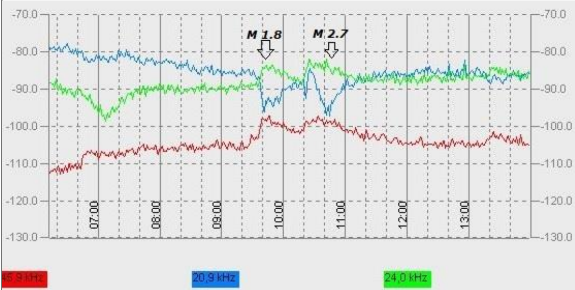
Two of many M class flares this month, June 12, 2014. Graph from A139 F Francione & C Re, Turin, Italy 45.9kHz (NSY) 20.9kHz (HWU) 24.0kHz (NAA)
