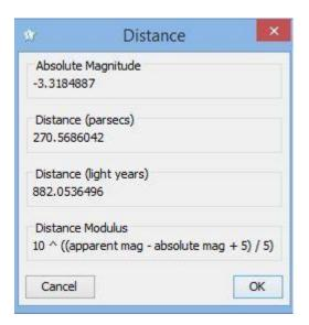
The distance will vary depending on the series used (visual, Johnson V, etc.), the range of data used to calculate mean magnitude and period. Also shown in the distance box is the distance modulus, the formula used to calculate the distance in parsecs.
