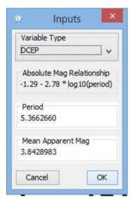
There is a drop down menu for variable type. At this time the only variable type supported for this particular Plug-in is DCEP. The next input is for the period. The default period is the period obtained from VSX. If you prefer, you can calculate the period for the current range of data that you have loaded by using DC DFT Standard Scan from the analysis menu.
