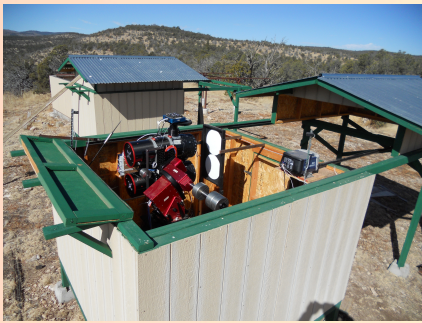
Figure 1: APASS-north installation at Dark Ridge Observatory, Weed, NM. Note the flatfield screens; projection lamps are on the ends of the telescopes.
