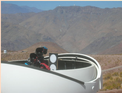
Figure 2: APASS-south installation at CTIO. This system uses the PROMPT-6 clamshell.
