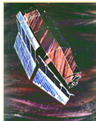
The second of NASA's High Energy Astrophysical Observatories, HEAO-2, renamed Einstein after launch, was the first fully imaging X-ray telescope put into space. The lifetime of the satellite was from November 1978 through April 1981.
