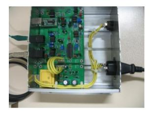
Figure 10 - SID Receiver circuit with internal capacitor and variable resistor
