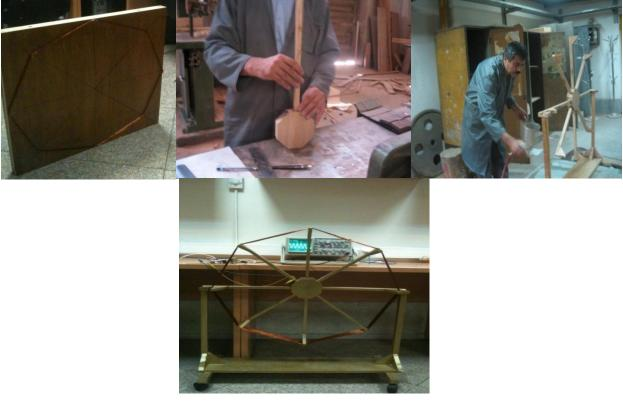
Figure 3 Different phases of building the octagon antenna: a. Building of the octagon wooden piece in the center of the loop shape antenna. b. Assembling and mounting the wood pieces around octagon loop shape.
