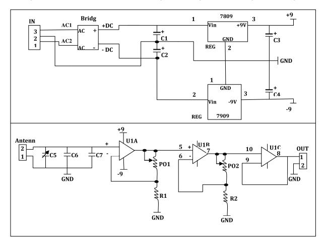
Figure 4 - Amplifying schematic circuit for octagon loop antenna
