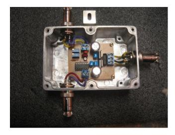
Figure 5 - Amplifier circuit is placed in a metal box general design from Percival Andrew, 2007
