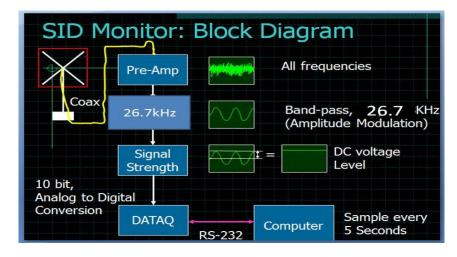
Figure 8- Block diagram of receiver with the internal capacitor/ resistor filter using the square loop antenna
