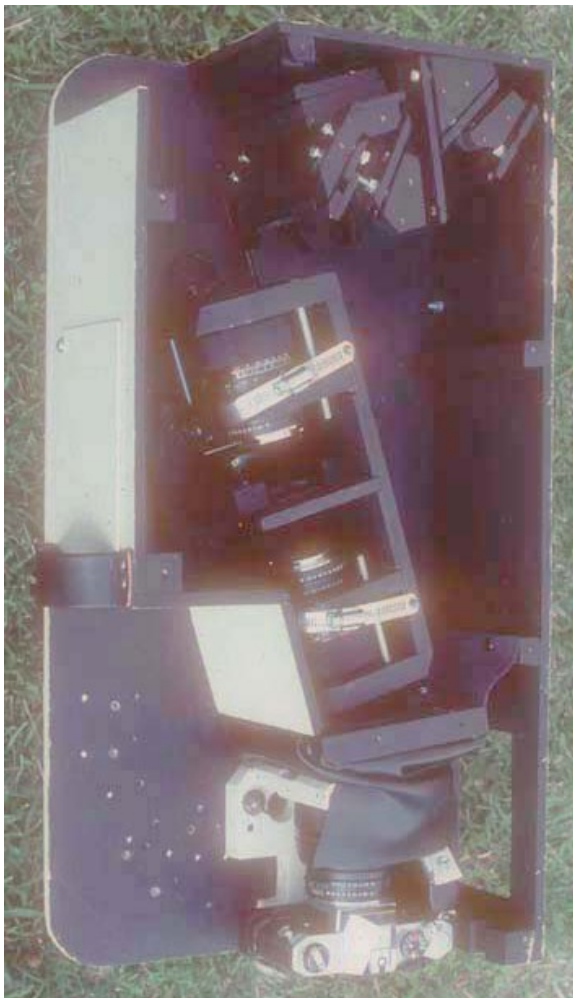
Figure 12. Inside Top View of Spectrograph Showing Slit Unit in Place. A Corner of Camera Support Is Set on a White Dot, Position # 1, for First Order. Seven Dots Mark All Positions.
