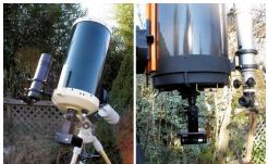
**Figure 1**. Optec SSP-3 and SSP-4 photometers on Grand View Observatory, Vixen (left) and Celestron (right) telescopes. Note the generous finderscopes - invaluable for time-efficient target acquisition.
