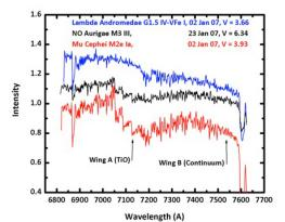
**Figure 3**. Spectra of 3 different class variable stars in wavelength region of Wing WA and WB bands taken with SBIG SGS spectrograph using ST7-XME CCD camera: lambda Andromedae (RS CVn, G8 III-IV); NO Aurigae (SRc, M3 III); and mu Cephei (SRb, M2e Ia). The TiO absorption bands are readily apparent in the Mtype stars.
