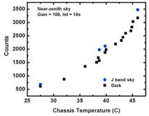
**Figure 4**. SSP-4 dark (squares) and J band sky (circles) counts versus chassis temperature:  $T = -40^{\circ}$ F, Integration time = 10 sec; Gain = 100.
