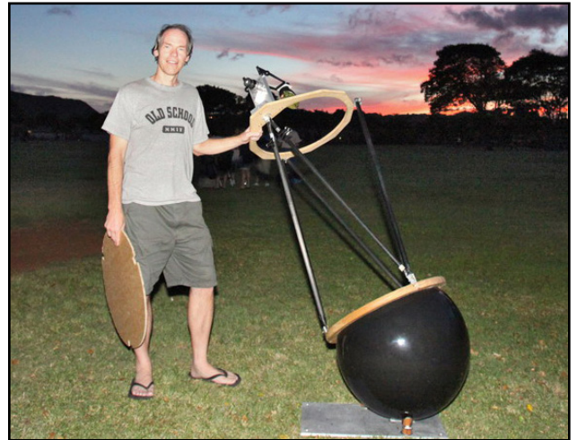
Mike Linnolt (LMK) with his homebuilt 20-inch f/3.6 sphere-mount Newtonian reflector.
