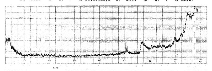
The above recording of 27 kHz atmospheric noise shows a sudden enhancement (SEA) starting at 0936 UT and reaching maximum four minutes later. By 1000 UT the disturbance of the ionosphere has ended. This record was made by A-17, Durban, Natal, Republic of South Africa.
