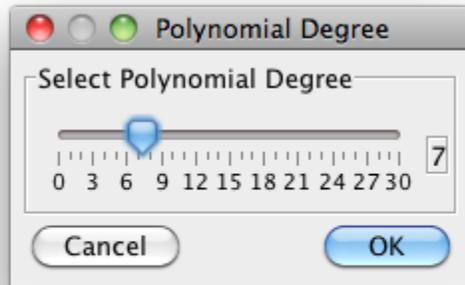
This is used to specify the number of degrees for the polynomial to be created, 7 in this case. Clicking the OK button creates the polynomial fit of the Visual series and adds a Model series as follows:
