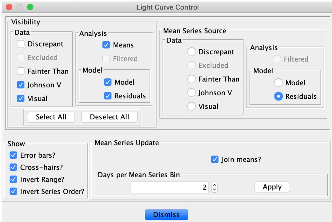
In addition, as shown above, if the `Residuals` mean series source radio button is selected and Days per Mean Series bin set to 2, as shown, the Plot Pane will look like this:
