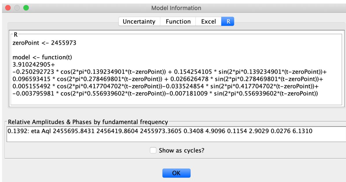
The model equations can be selected and copied with the mouse (via manual selection or select-all/copy keyboard shortcuts) and used as part of a script. For example, from the dialog above, the R Fourier series equation:
