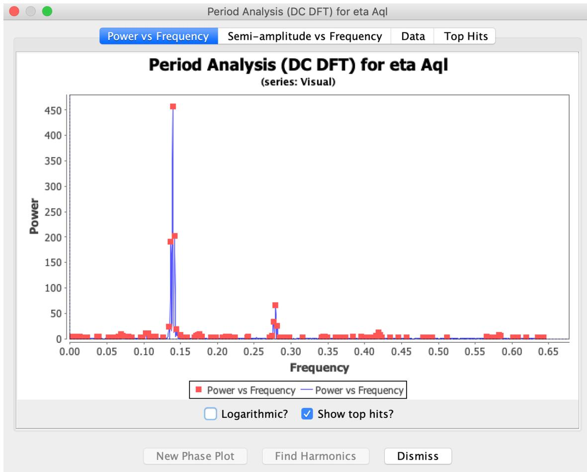
By default, the `Power vs Frequency` plot (sometimes called the “power spectrum”) is shown. Notice that `Show top hits?` is checked here, again, by default. The small brightly colored squares correspond to “top hits,” those frequencies/periods at the peaks of the plot (those with highest power value). These are the best candidates for the actual frequency (period).
