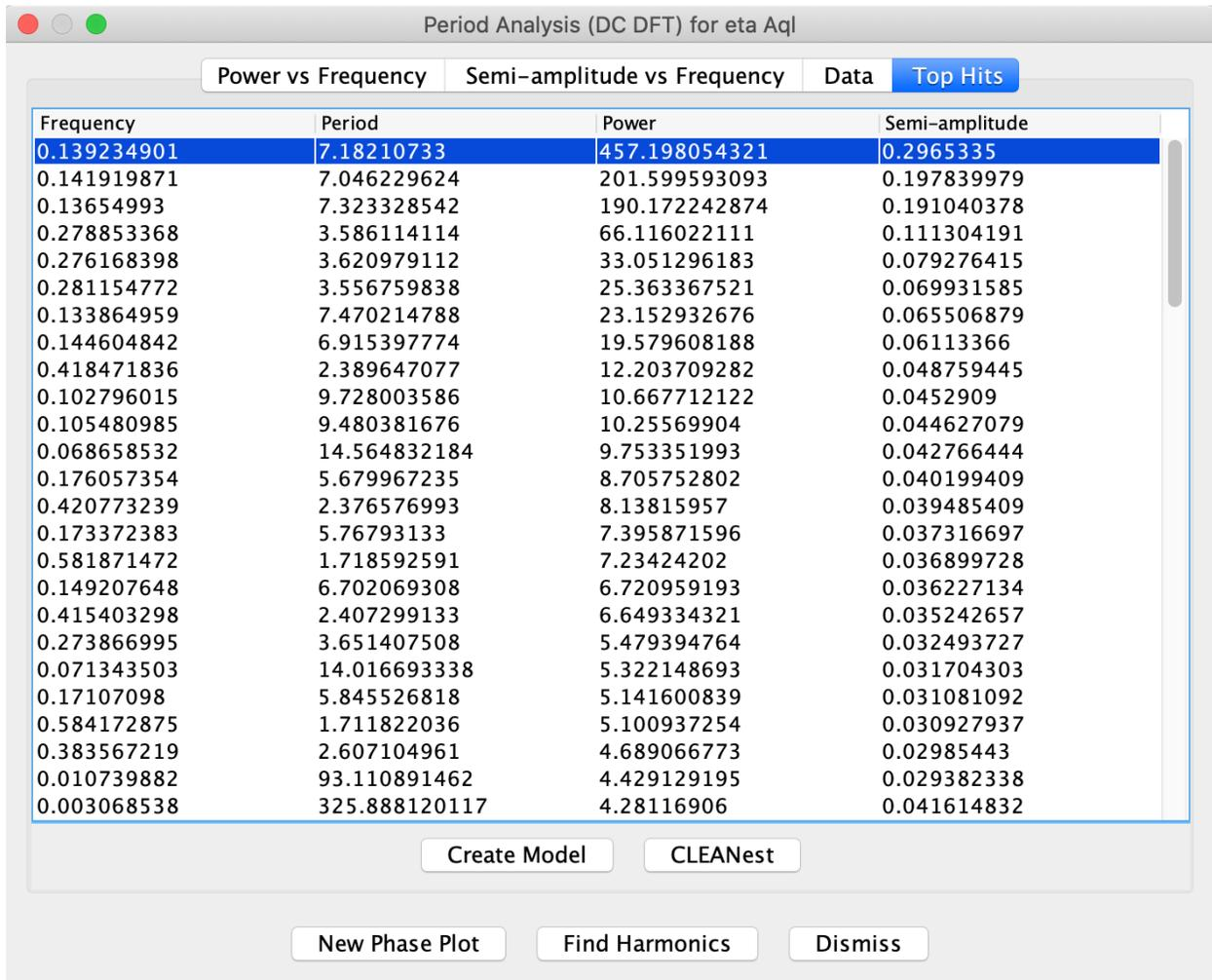
Clicking the New Phase Plot button with the shown top-hit selected will result in the phase seen earlier in this section.
