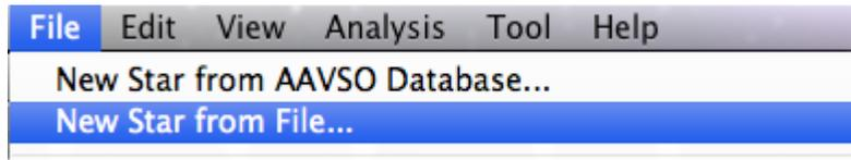
The file chooser that opens defaults to the observation source “Download or Simple”. Such files must conform to one of two formats:
