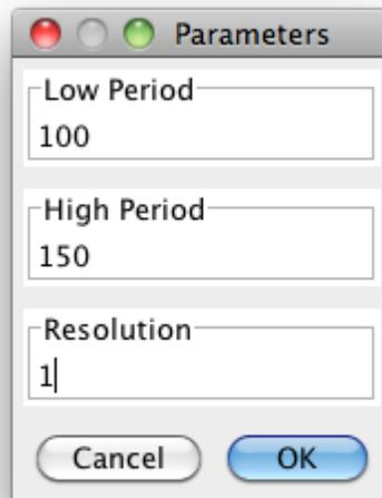
The DCDFT with Frequency Range option populates the dialog with an initial frequency range and resolution as described for Standard Scan above.
