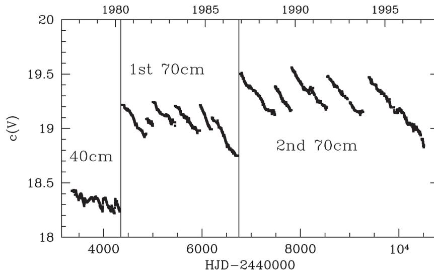
Figure 1. Variations of the instrumental coefficient in the  $V$  band for the Swiss telescope at La Silla Observatory. The changes of telescope and the aluminum coating of the mirror, as well as the series of cleanings of the mirrors (telescope and/or photometer) are clearly visible (for more details, see Burki *et al.* 1995).
